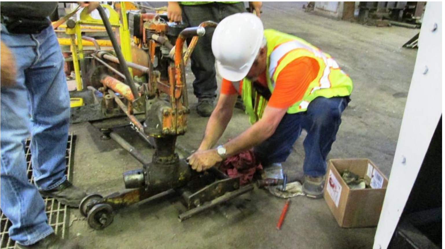
Ed replaces the keeper pin on the bolt machine at the socket
